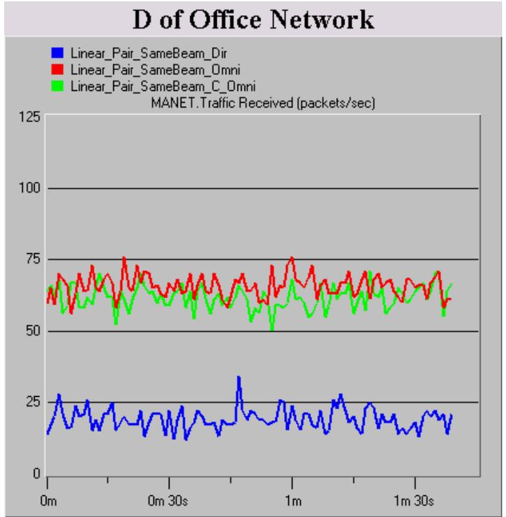
(b) Packets received by receiver node D vs. time
