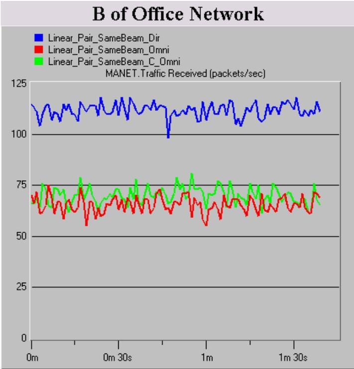
(a) Packets received by receiver node B vs. time
