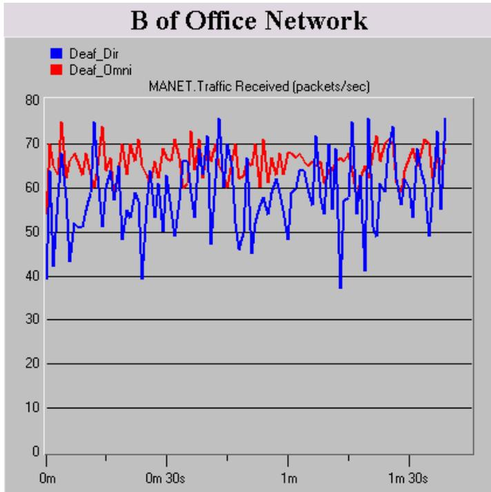
(a) Packets received by receiver node B vs. time
