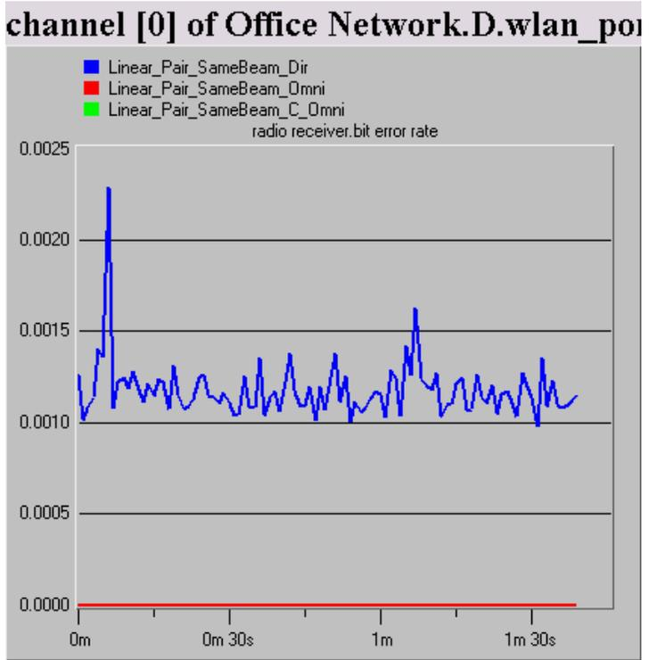
(d) Bit Error Rate at receiver node D vs. time
