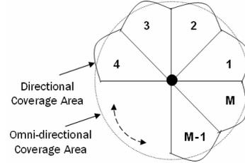
Figure 3. The antenna model
