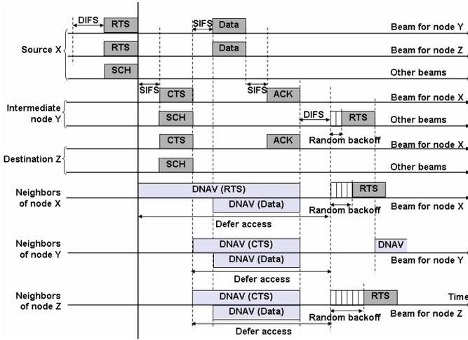
Figure 1. Basic operation of MMAC-NB
