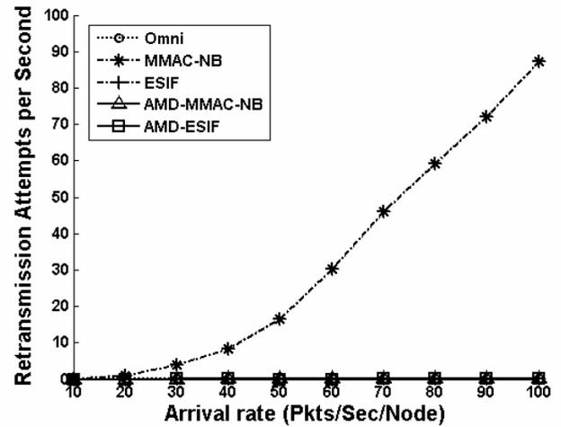
Figure 6. Retransmission attempts made by transmitting nodes in topology 1
